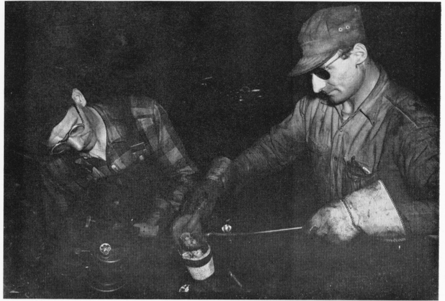
Here John Jacewicz and Henry Carisio are making up hoisting cables. Henry is pouring babbit into the thimble. Babbit is tough, holds the cable firmly on the socket. The Electrical Department has sole responsibility of maintenance of cranes from stem to stern.
